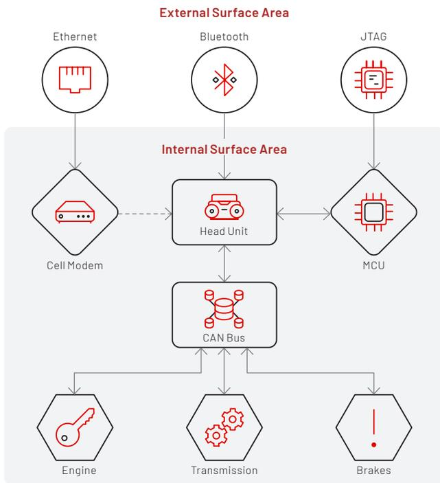
FIGURE 1. Sample threat model of a connected car.
