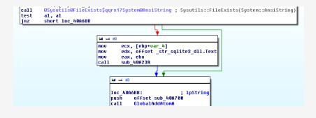
**Figure 5:** IntelRS.exe sleeps until global atom is set and sqlite3.dll is present
